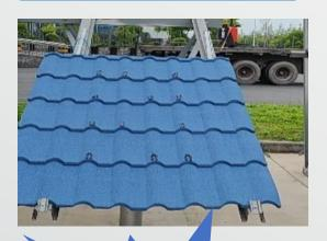
When roof slope is ≥ 25°, the rear area of module needs to be bonded with double-sided foam tape for preventing from slipping and/or shifting.
